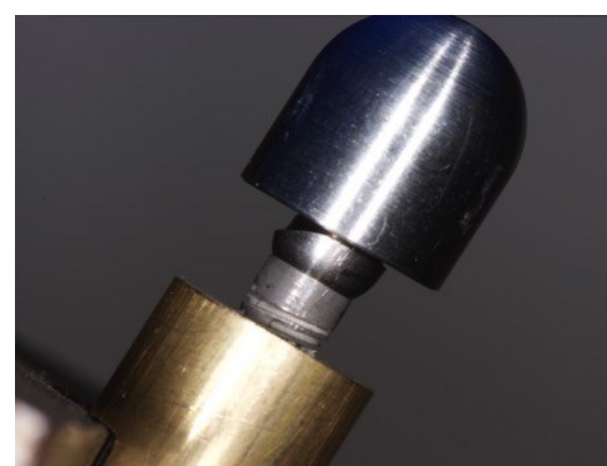
Fig. 1: test sample Following ISO 14801
